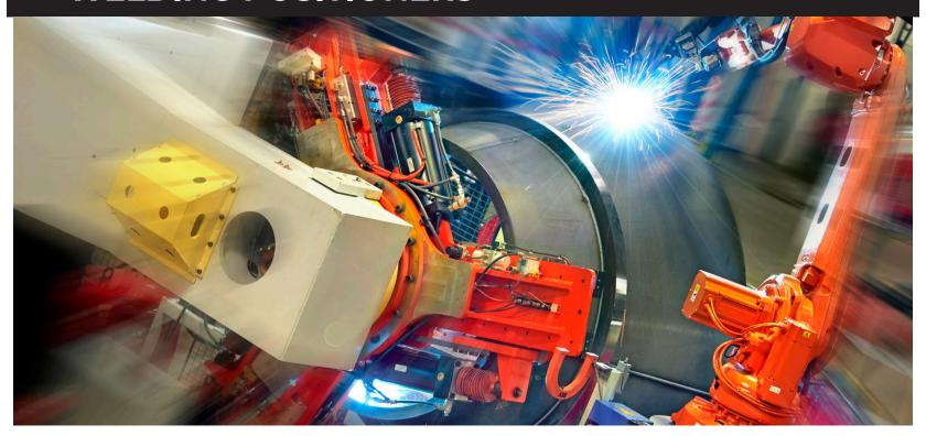
Robotic welding positioners are offered in a large range of models and capacities and are one of MWES' most popular welding capabilities. Our welding positioners allow robotic manipulators to move weldments in one or more axes. This gives the robot precise positioning for optimal welding for any type of components from simple to complex geometries.
