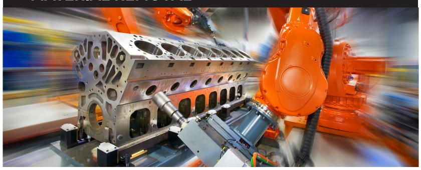
Automating metal removal, degating, and deflashing of castings, and even material handling applications, can overcome a shortage of workers that many foundry and casting firms struggle with. Using cutting-edge technologies including the latest in robotic technology and machine vision, MWES can achieve desired casting finishing production and quality goals while producing more consistent parts while reducing reliance on manual labor.
