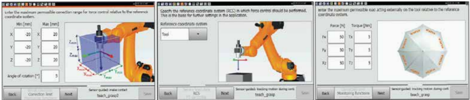
Snapshots for setting up a Force/Torque application on the teach pendant
