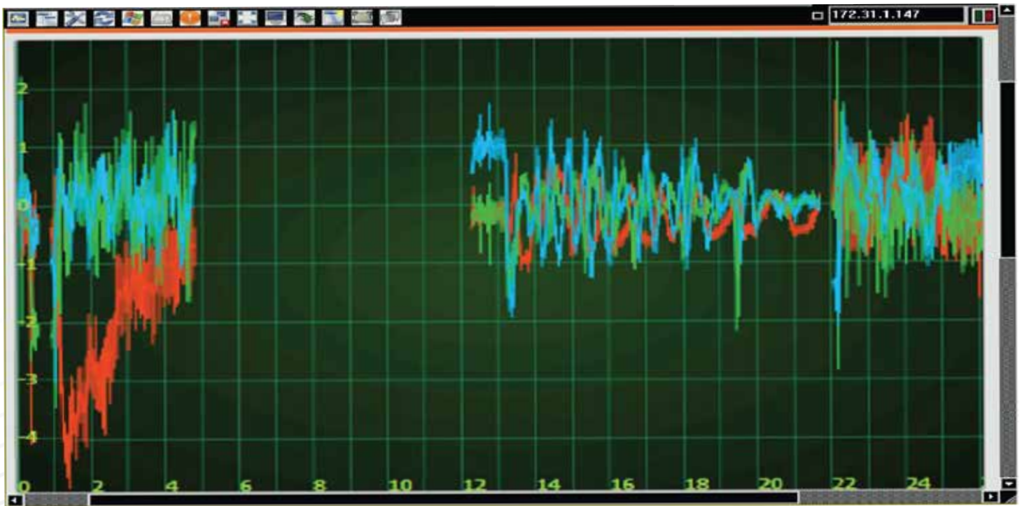
A graph of the forces and torques that is generated by the Force/Torque Software
