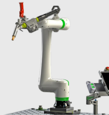
Closer View of Cobot with Patented IMITE EOAT Mounted to Arm
